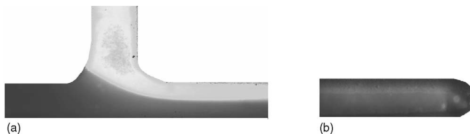
Fig. 8. Visualization of the mixing in the reaction channel by LIF measurement: (a) microchannel inlet; (b) microchannel outlet. The white fluid represents the fluorescent dye; the black fluid the acidic solution. Flow rate of the feed streams of 2 \mu\text{l min}^{-1} .
